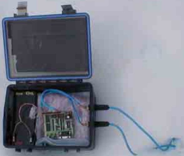
Basic stamp data logger w/ 7 Amp-Hour battery
